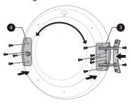
On the appliance cabint, unscrew 2 screws and remove the door catch **5**. Reassemble it on the opposite side of the door.
