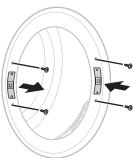
7 Reassemble the door on the cabinet using the screws removed in step 1. Make sure that the door opens, closes and latches properly.
