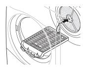
Seat the front of the rack securely on the inner door rim and the back of the rack on the rim at the back of the drum.
