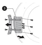
3 Remove the 3 screws from the door latch assembly 4 which is mounted between the door and the hinge assembly. Remove the screw in the door latch.
